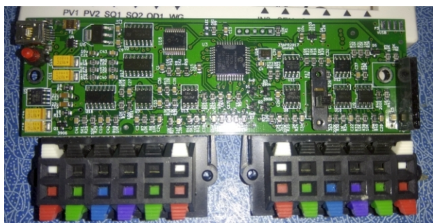
Figure 2: A view of the Internal Circuit Board of the ExpEYES-17 kit.
