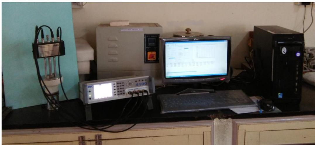
Fig.1 Photograph of automated LCR meter setup for measurement of dielectric constant of contaminated and reclaimed soils
