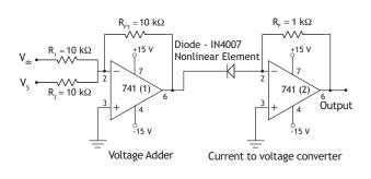
Figure 2: A diagram of a circuit designed to study the nonlinearity of a *PN*-junction diode. Two 741 general purpose operational amplifiers with a *PN*-Junction diode IN4007 are used in the circuit. Output of an inverting voltage adder is applied across a *PN*-junction diode. The output voltage of the circuit is proportional to current passing through the *PN*-junction diode.
