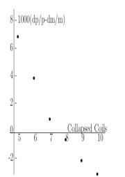
Figure 3. Sign change of (dp/p -dm/m) occurs between coils 7 and 8 at maximum speed
