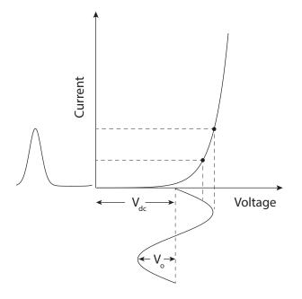
Figure 1: A schematic showing an exponential dependacnce of current on the forward bias voltage across a *PN*-junction diode. A variation of diode current for a sinusoidal bias voltage of amplitude  $V_o$  with a dc offset  $V_{dc}$  is also shown.
