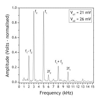
Figure 6: A frequency spectrum of the output voltage waveform shows the sum ( $f_1 + f_2$ ) and difference ( $f_1 - f_2$ ) frequency generation. Second harmonics of frequencies  $2f_1$  and  $2f_2$  corresponding to each input voltage waveforms are also produced.
