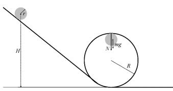
Fig. 1 Solid sphere on a loop-the-loop.
