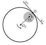
Fig. 2. Description of the rolling of the ball as superposition of the rotation with respect to point  $O_2$  with angular speed  $\omega_2$  and rotation with respect to the point  $O_1$  with the angular speed  $\omega_1$ . Instantaneous velocity of the rolling ball at the point O is equal to zero and angular speed with respect to this point is  $\omega = \omega_1 - \omega_2$ .
