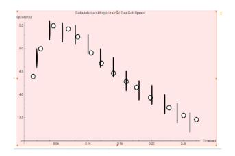
Figure 1 displays both the experimental (vertical bars) and calculated (circles) values for the top coil speed as a function of time. The experimental data point is in the center of the vertical line, their maximum (top) and minimum (bottom) values display only 1/2 their uncertainty which was given as  $\pm$  0.4 m/s
