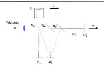
Figure 2. Set up for the Michelson – Morley experiment after being rotated through  $90^{\circ}$ .
