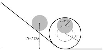
Fig. 3. The initial position and the position of the ball at the highest point for 2r=R. Dashed line is a trajectory of the center of mass.
