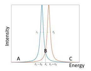
Figure 3. Profiles for the emission and absorption lines. Resonance fluorescence of  $\gamma$  – rays will occur only if the two profiles overlap considerably.
