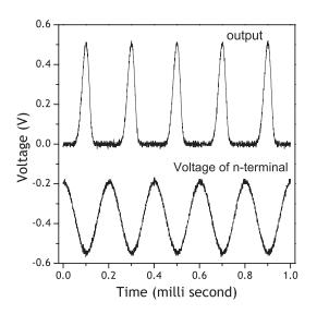
Figure 3: A plot showing an applied sinusoidal voltage across a PN-junction diode (lower plot). Output voltage  $V_t$  (upper plot) is linearly proportional to current passing through the diode. It is clearly shown that a sinusoidal input voltage gives rise to a non-sinusoidal output voltage due to the intrinsic nonlinearity of the diode.
